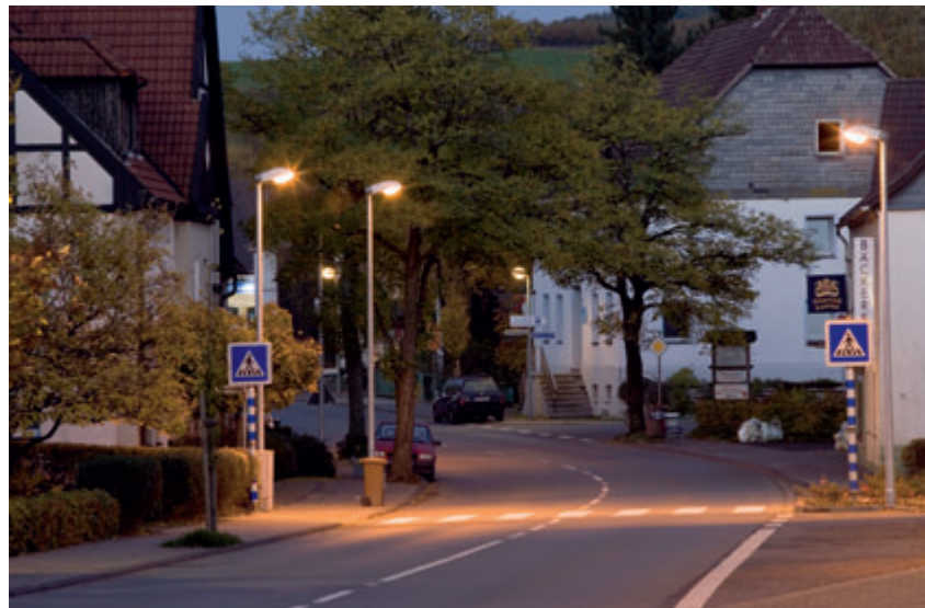
Fig. 17: Illuminating pedestrians from the side in the direction of travel (positive contrast); “h” is the mounting height of the luminaire.
